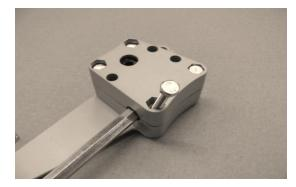
Place large plate on opposite side to which you took it off, drop bolts through. Turn unit over carefully and tighten bolts with the nuts you removed earlier.
