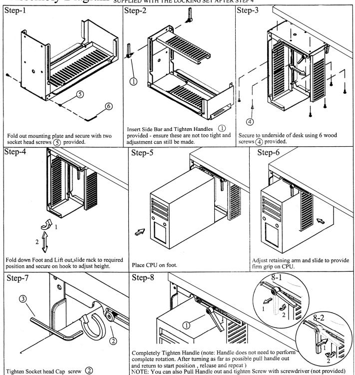
Please note: Illustration is for a left hand side application, if right hand is required please turn the CPU holder around as appropriate.
